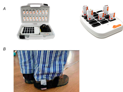
Figure 3. Gait analysis device. (A) Consensys Bundle Development kit; (B) The IMU sensor-wearing part.
