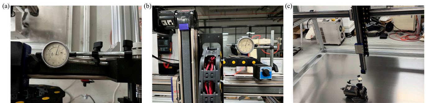
Figure 6. The testing process for repeat positioning accuracy: (a) X-axis; (b) Y-axis; (c) Z-axis.
