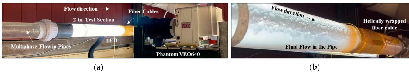
Figure 3. (a) Pictures of the testing section with the helically wrapped yellow fiber cables, and the high-speed camera taking videos. (b) A closer look at the wrapped fiber cable.
