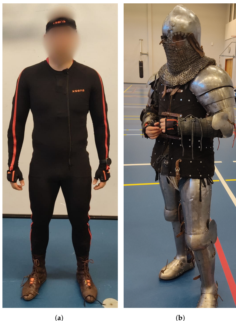
Figure 1. The XSENS MVN Link suit with 23 IMU sensors: (a) the combatant wearing the IMU suit; (b) the combatant in full armor on top of the IMU suit.
