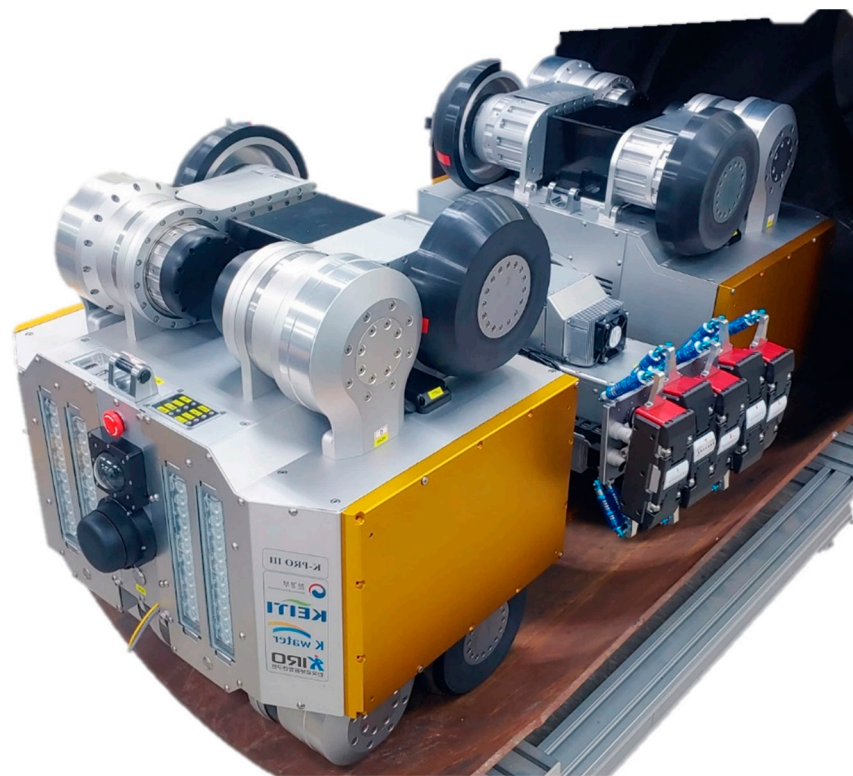
Figure 4. Developed in-pipe inspection robot.
