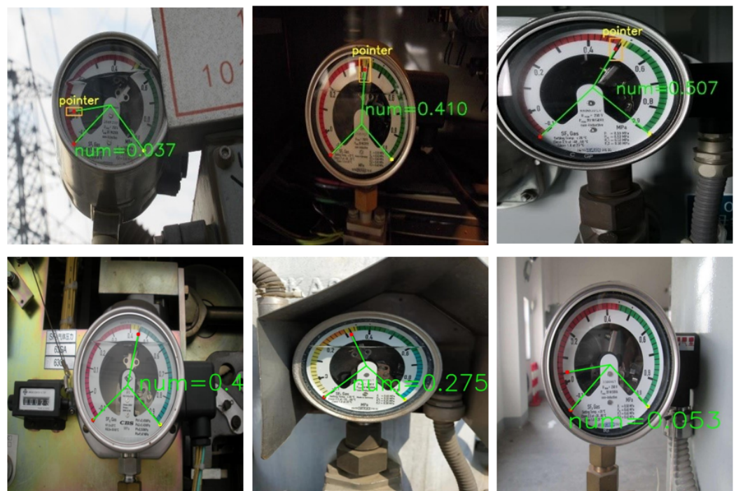
Figure 11. Actual industrial application examples of meter reading in the grid industry.
