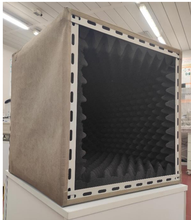
Figure 3. Picture of the shielding anechoic chamber.
