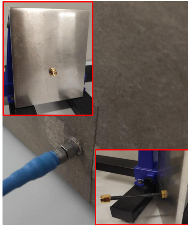
Figure 2. Picture of rear side of the chamber, with the detail of the panel connector in the insets.
