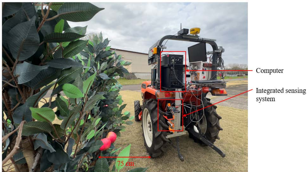
Figure 7. Outdoor experimental setup for obtaining static depth values of apples under different light conditions in an artificial spindle orchard.
