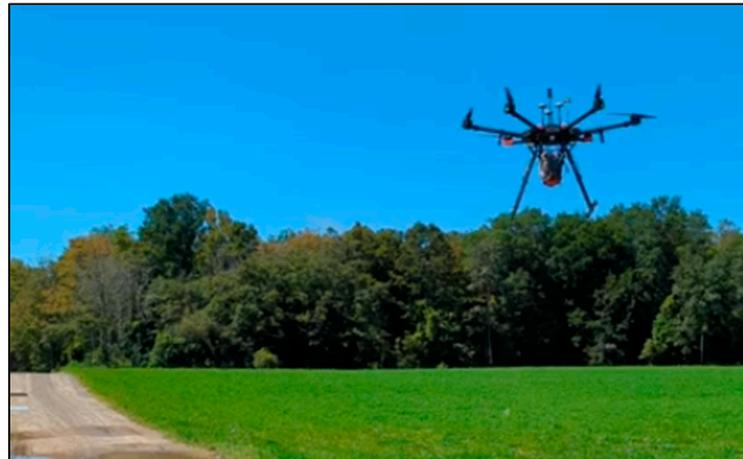
**Figure 2.** The UAS imagery collection platform used for this study, a DJI Matrice 600 Hexacopter. On board is a 272-band imaging spectrometer, a five-band multispectral imaging sensor, LIDAR, thermal imaging sensor, high resolution RGB imaging sensor, a downwelling spectrometer, and GPS navigation equipment.
