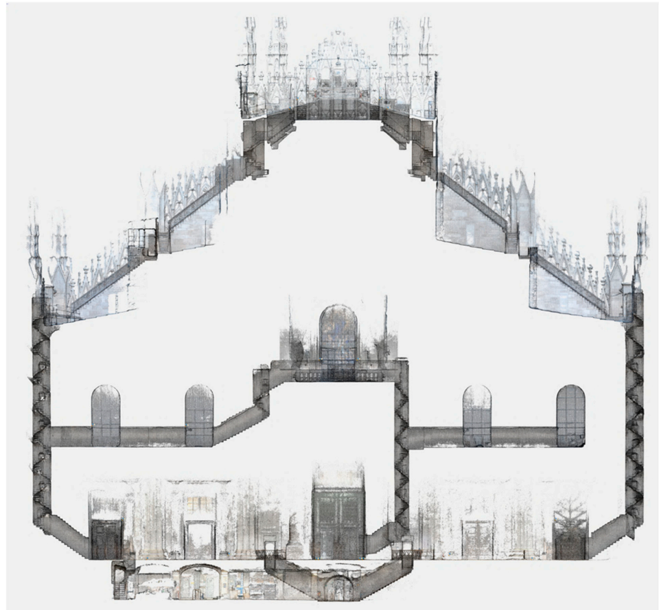
Figure 22. The elevation view of the point cloud generated from the Ant3D survey of Milan's Cathedral façade's narrow spaces and corridors. The image was extracted from a prior publication; additional details on the processing can be found at [22].
