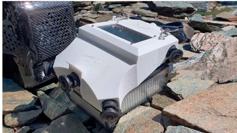
Figure 16. A picture of the second version of the prototyped instrument. The picture shows the probe in the front, the backpack that houses the PC, and the battery on the back on the left.
