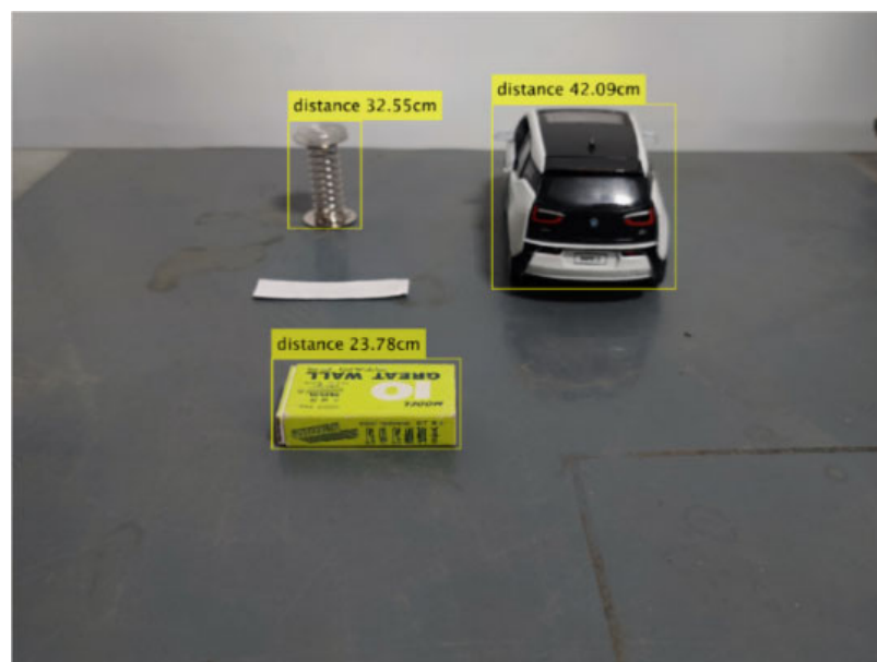
Figure 12. Obstacle area division (where the yellow box is the detected obstacle area and the upper number is the distance from the obstacle to the camera).
