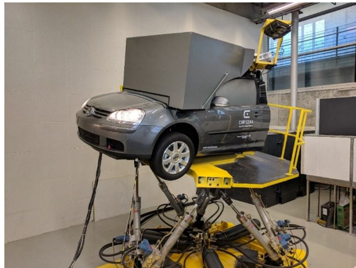
Figure 2. Driving simulator on a hexapod test rig at Technische Hochschule Ingolstadt [20].
