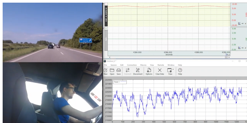
Figure 4. Acquired data during on-road measurement: street view, driver view, and sensor signals (( top ) gold standard ( bottom ) custom sensor signal).
