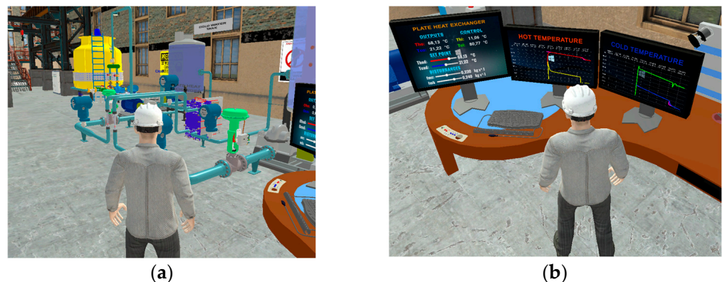
Figure 7. Virtual process environment: (a) industrial environment with heat exchanger and (b) monitoring and control area.
