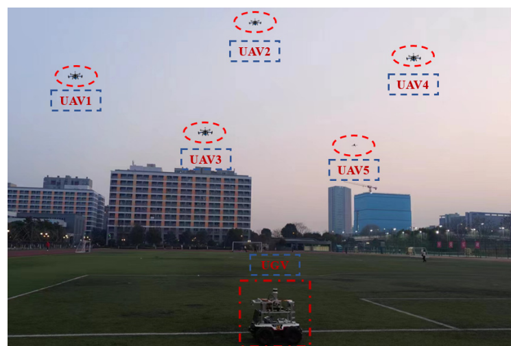
Figure 7. The cooperative localization scenario between UAVs and UGV based on relative distance constraints on outdoor campus playground.
