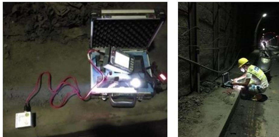
Figure 20. Field monitoring for blasting vibration.
