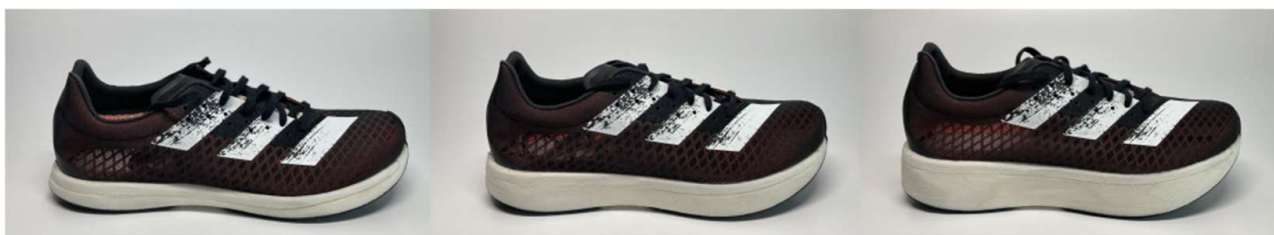
Figure 1. Shoe conditions displayed by stack height in ascending order, from left to right (25 mm, 35 mm, 45 mm).
