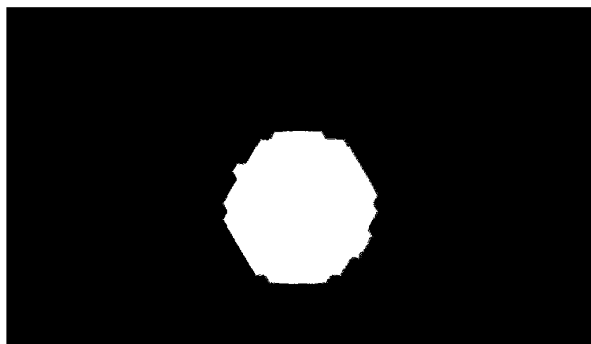
Figure 7. Saturation mask in which the zero S pixels are represented in black.
