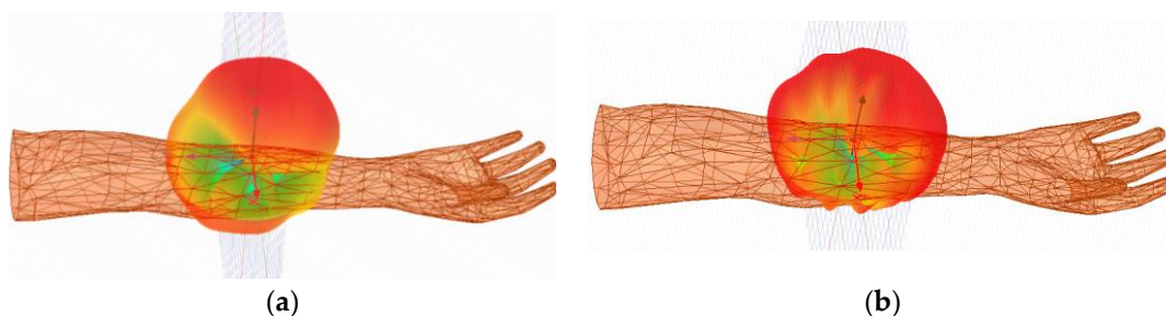
Figure 16. Antenna three-dimensional radiation direction map: (a) 1.4 GHz, (b) 2.45 GHz.
