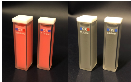
Figure 1. Example of filled cuvettes with IL and red ink (left) and black ink (right).
