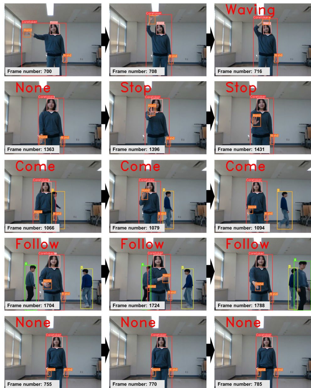
Figure 14. Typical instances of 5 categories of gestures recognized in real time within an authentic environment are showcased, utilizing the gesture recognition network integrated into RFIS. Note: the use of a low-resolution camera for computational efficiency somewhat compromises the image quality.
