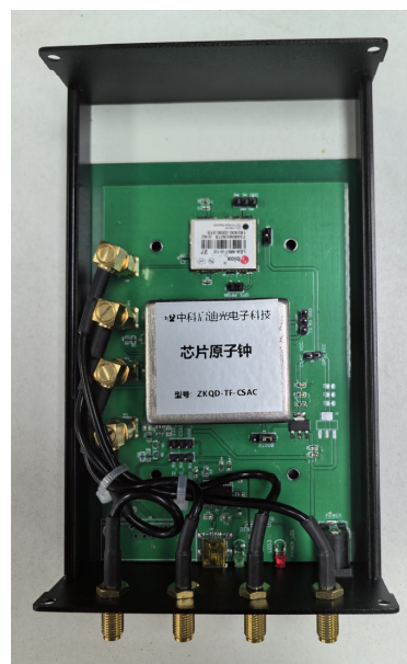
Figure 5. An example of the ZKQD-TF-CSAC embedded GNSS receiver, supplied by ZhongkeQidi Optoelectronic Technology (Beijing, China). Due to commercial secrets, we cannot show the newest version of this receiver. For more information, please see [38].
