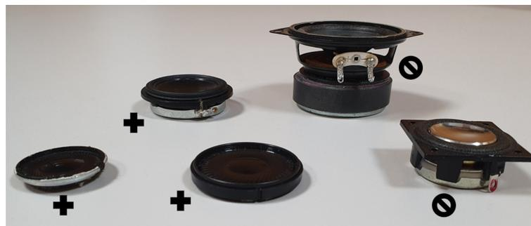
**Figure 2.** Comparison of the badly shaped transducers (crossed circles) and the design of the proper shape for the array loudspeakers (plus signs).
