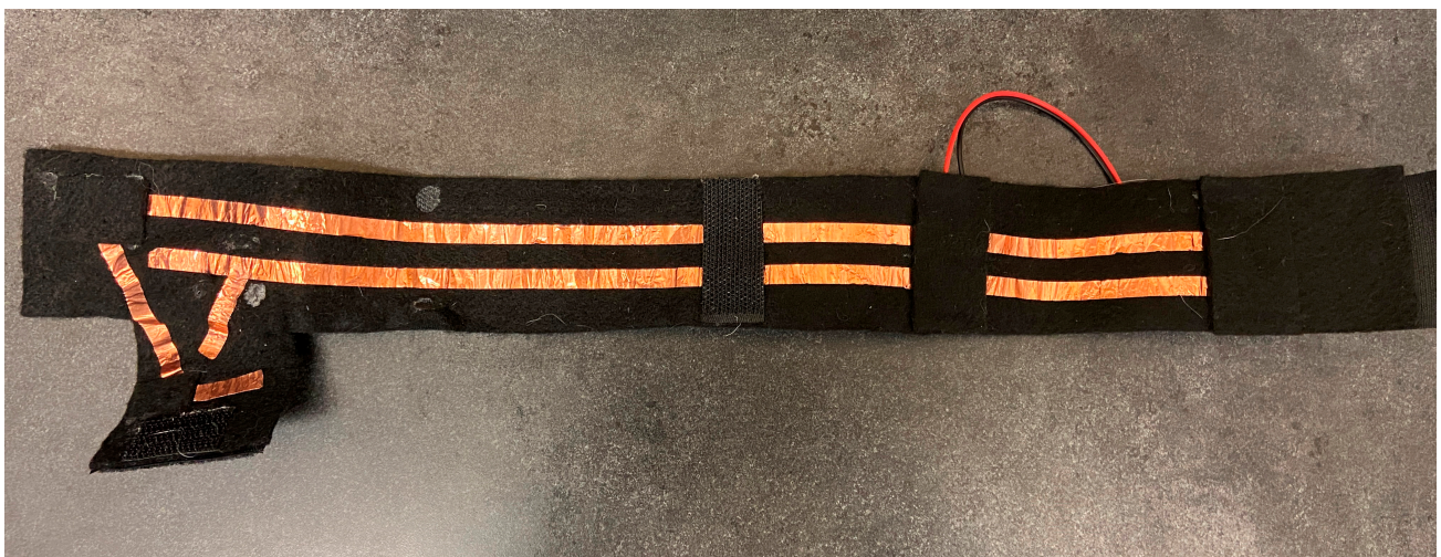
Figure 3. Conductive wrap to provide power to the vibration liner without donning the socket. The arrangement of the copper tape aligns with the contact points on the liner when wrapped around the liner.
