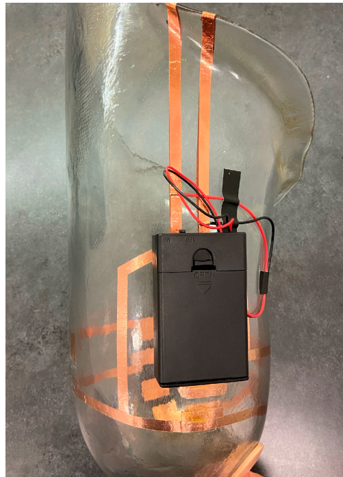
Figure 2. Anterior view of the final socket prototype with a battery holder attached. The arrangement of the copper tape aligns with the contact points on the liner when the socket is donned.
