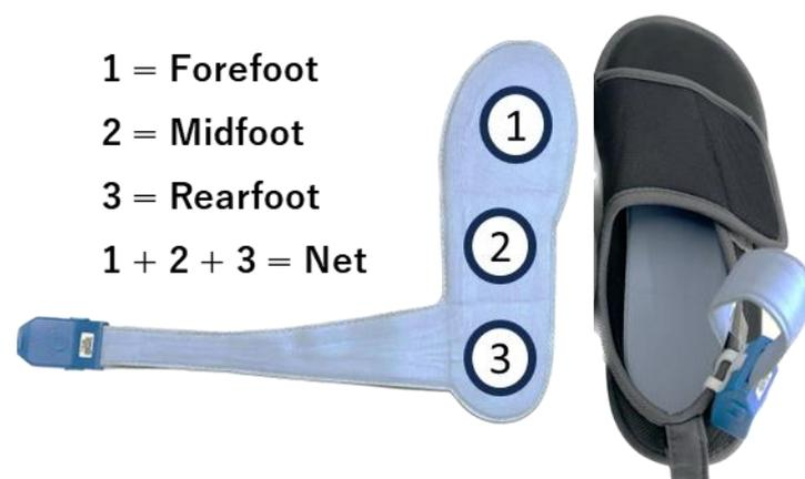
**Figure 2.** Overview of the three-sensor plantar force measurement insole device. Three sensors are inserted into a 3-mm-thick shoe insole. The insole is inserted in a commercial Velcro shoe, and the data acquisition unit is fixed using an attached clip on the shoe.
