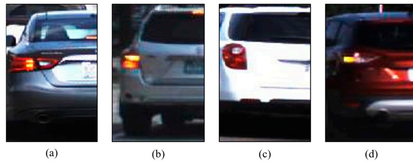
Figure 11. Examples of 4-class data for individual taillight classification: (a) B (brake light only); (b) BL (brake and turn signal light on); (c) O (brake and turn signal light off); (d) OL (turn signal light only).
