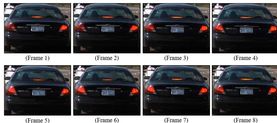
Figure 4. Example of brake light and turn signal using the same unit.
