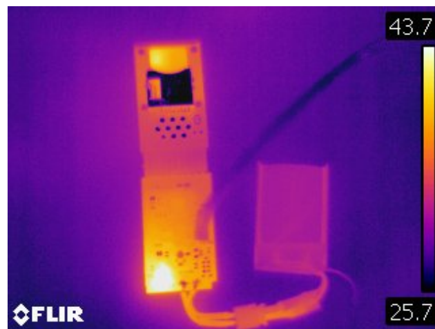
Figure 5. Thermal image of sensor charging process, highlighting the STNS01's role as a BMS.
