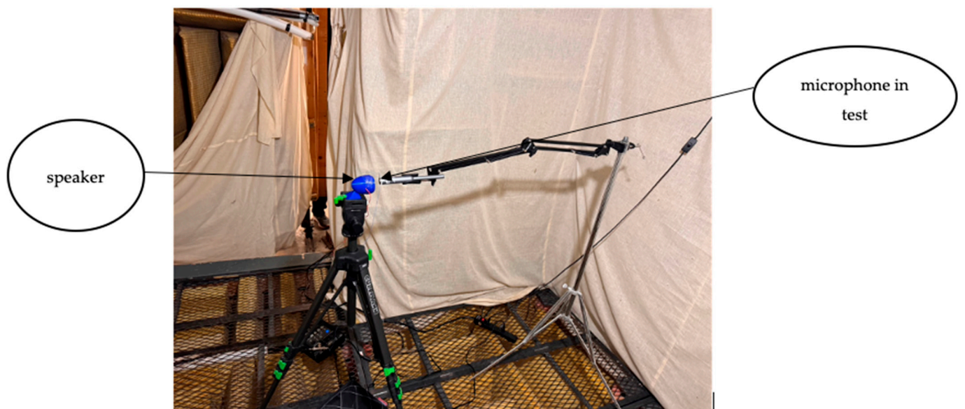
Figure 1. Test 1 setup in the anechoic chamber.
