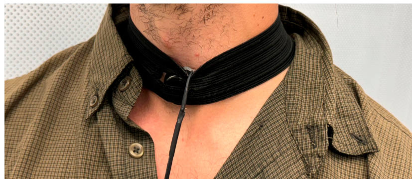
Figure 2. Subject position and microphone placement for tracheal breathing sounds recording (Test 2).
