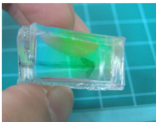
Figure S4. A photograph the PDMS stamp after detaching from the holographic glass grating (master grating).
