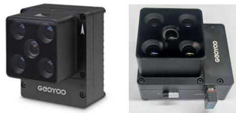
Figure 2. MS400 series multi-spectral camera.
