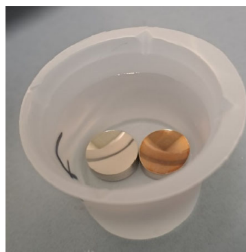
Figure 16. Two stainless-steel mirrors, one grafted and the other not grafted.
