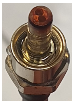
Figure 11. Grafting of NR on the end of a two-way metallized optical fiber.
