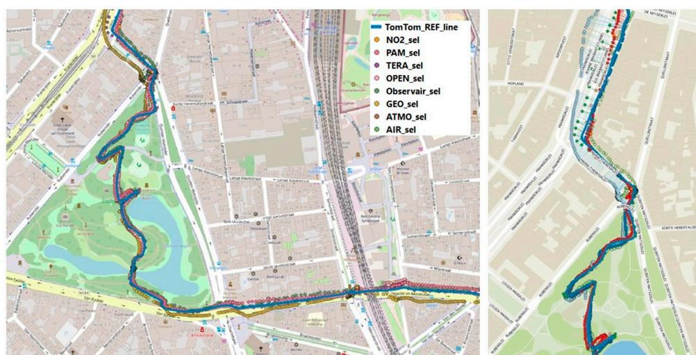
**Figure 7.** (Left): GPS tracks of the considered sensor systems (dots) and reference GPS track (blue line). (Right): Accuracy calculation by means of horizontal distance to reference GPS track (blue line).
