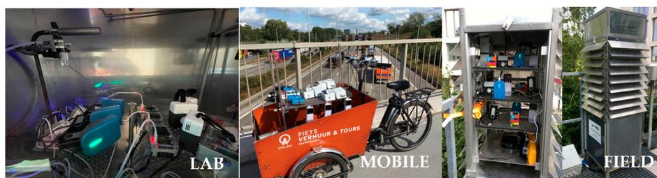
**Figure 2.** PM exposure chamber in the lab (left), mobile field test with cargo bike (middle), and field co-location campaign at an urban background monitoring station (right).
