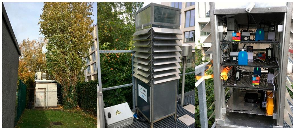
**Figure 8.** Location of the exposure shelter on top of R801 urban background monitoring station (left), detail of the exposure shelter (middle), and positioning of the sensor systems at the different platforms inside the shelter (right).
