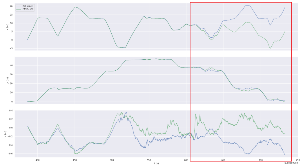
Figure 10. XYZ Components of Trajectory Estimation for FAST-LIO2 and RIL-SLAM. The red framed section indicates the part of the drift in FAST-LIO2.
