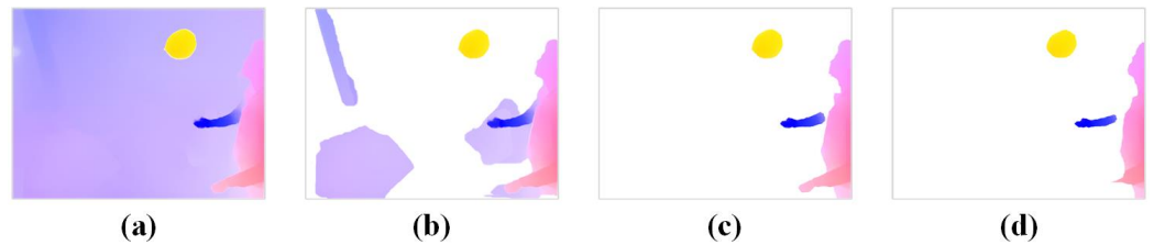
Figure 7. Iterative removal of camera self-motion flow using optical flow residuals. (a) Original dense optical flow. (b) Number of iterations = 5. (c) Number of iterations = 7. (d) Number of iterations = 9.
