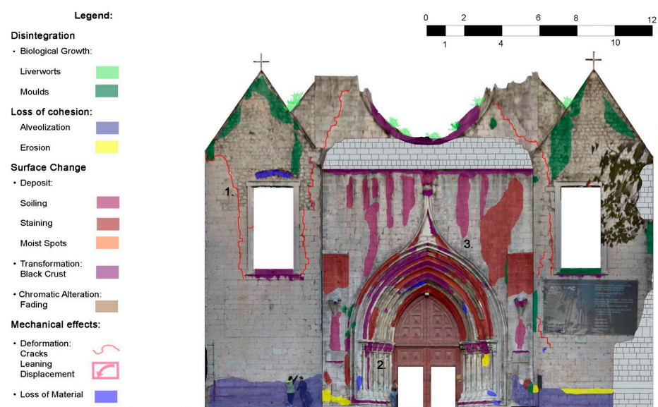
Figure 7. Example of damage pattern for the main façade before conservation and restoration works.
