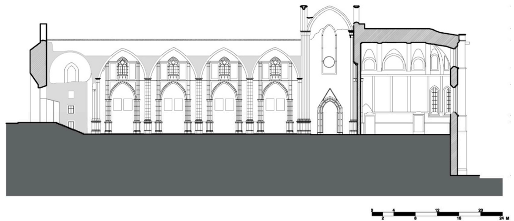
Figure 4. Section view of the interior (ee') of the church's nave featuring the arcades.
