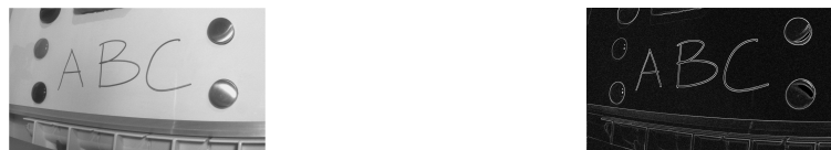
Figure 10. Application of the Sobel filter (original image on the left and the processed image on the right ).
