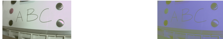
Figure 9. Application of the RGB/YCbCr conversion (original image on the left and the processed image on the right ).
