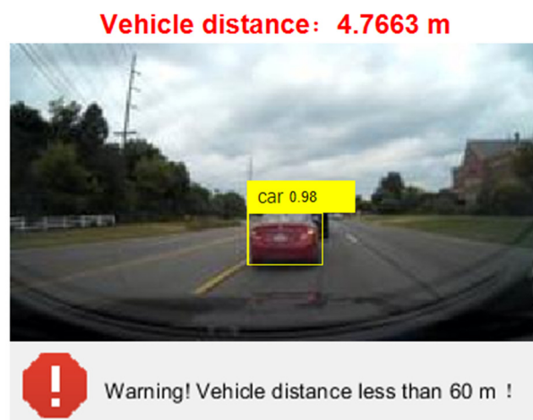
Figure 14. Capture vehicle image information (when the current rear distance is less than 60 m or the left and right distance is less than 1.5 m).
