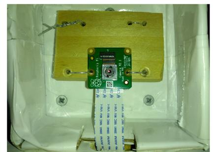
**Figure A4. Traffic sensor hardware.** LEFT: The hardware is placed into a separate wooden box on top of the hive and separated from the hive by an inner hive cover. RIGHT: A Raspberry Pi v2 camera (8 megapixel,  $1080 \times 1920$  pix resolution) is connected to the Raspberry Pi computer; the camera looks down on the landing pad of the hive from the top of the second super in Figure A2.
