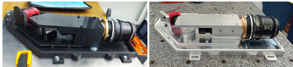
Figure 4. The 3D-printed (left) and aluminum CNC-machined (right) versions of the prototype.
