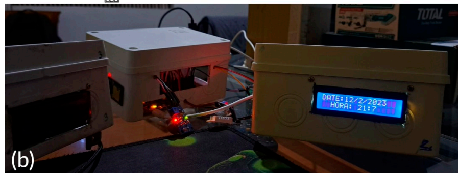
Figure 3. (a) Scheme of the portable analyzer for CO 2 monitoring; (b) analyzer finished.
