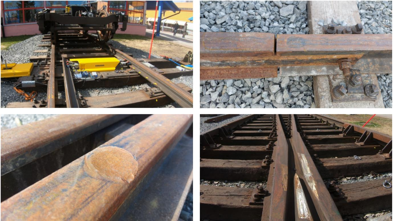
**Figure 2.** Experimental setup with track discontinuities and defects (cf. Figure 1). Point machine with bogie (upper left), joint X (upper right), squat D (lower left) and crossing (lower right).
