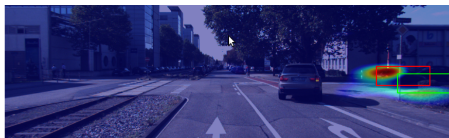
Figure 9. Contrastive explanation using the D-RISE method. The red bounding box represents the predicted bounding box, and the green box shows the contrastive example. The heatmap highlights the regions with higher activations in red.
