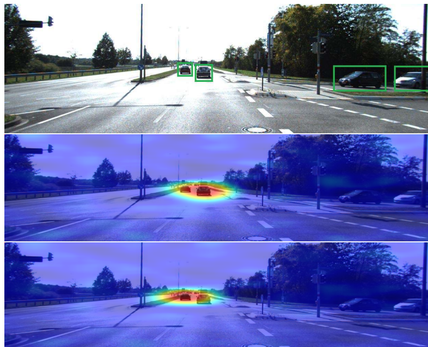
Figure 10. YOLO explanations obtained for two different objects in the same image. The bounding boxes are marked in green. Saliency maps highlight in red the regions with higher activations.
