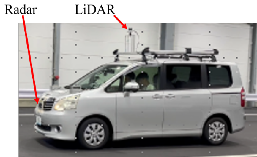
Figure 5. Sensor configuration of the experimental vehicle for data acquisition of the JARI and Tokyo data set. LiDAR and radar sensors were attached to the top of the vehicle and in the front license plate position, respectively. The LiDAR sensor employed in the proposed method is the Ouster LiDAR with 64 vertical channels. Precise calibration was carried out to ensure accurate data collection.
