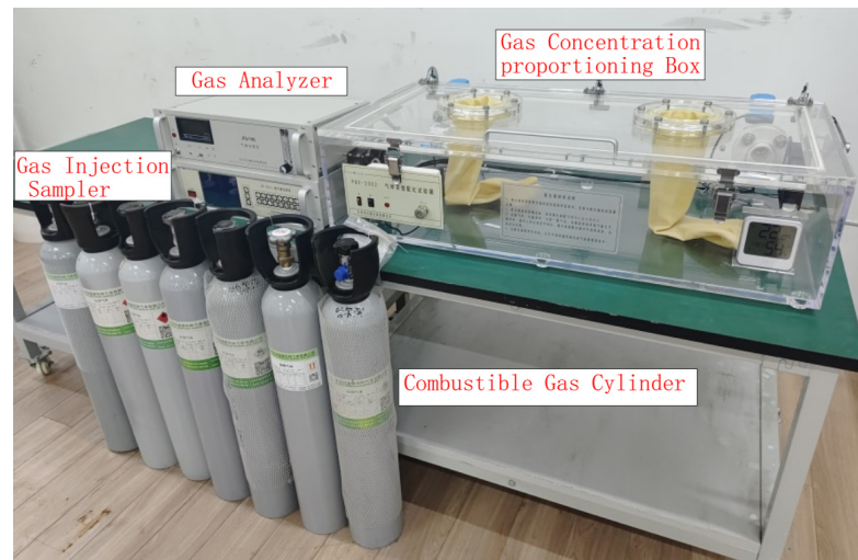
Figure 6. Methane gas concentration proportioning device diagram.
