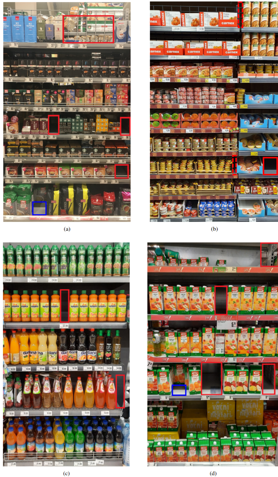
Figure 7. Examples of OOS detection results. The top row (a,b) displays the successfully analyzed images, whereas the bottom row (c,d) shows images with partially inaccurate results. The detected OOS instances of the normal and front classes are marked with red and blue bounding boxes, respectively. In (b), the dashed bounding boxes represent the OOS instances that were detected by the model but discarded after the post-processing was applied.
