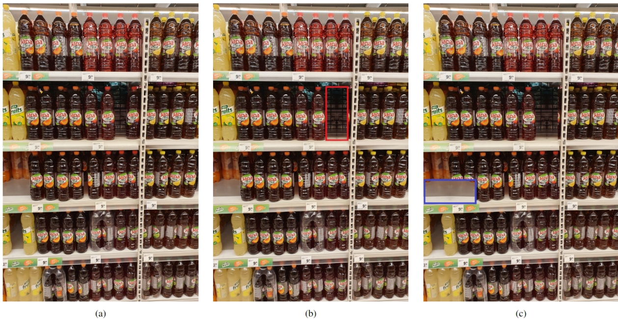
Figure 5. Example of the OOS mirroring procedure. In the first iteration, the proposed OOS mirroring technique is applied to (a) the original image to produce (b) the first augmented image. In the second iteration, the augmentation technique is applied to (b) to produce (c) the second augmented image. For each iteration, the newly extended OOS instance is marked with a color-coded rectangle, where red and blue colors represent normal and front classes, respectively.
