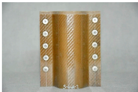
Figure 7. Glass-fibre-reinforced polyetherimide (PEI) absorber—WS-PEI.
