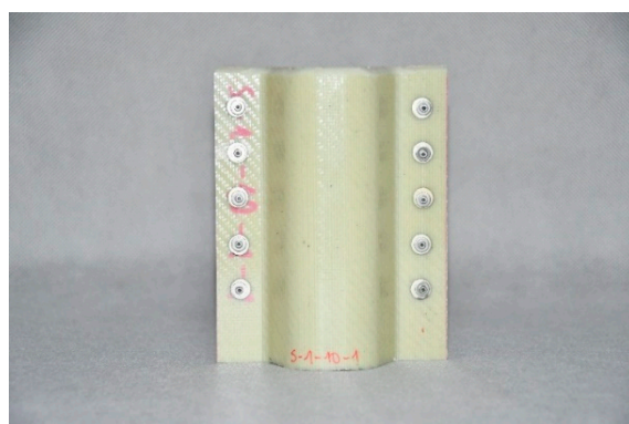
Figure 8. Glass fibre polyamide 6 (PA 6) absorber—WS-PA6.
