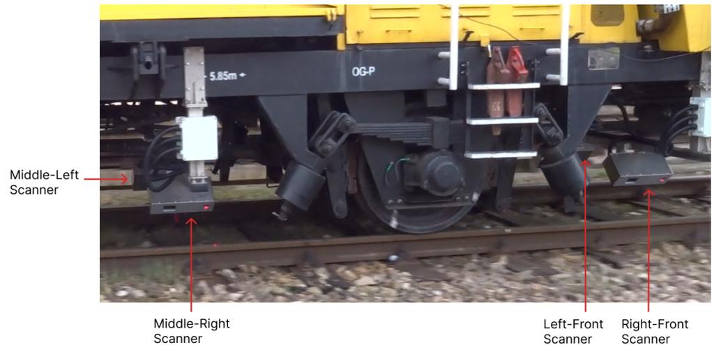
**Figure 2.** Four of the six rail-geometry-measuring module scanners attached to a rail maintenance vehicle.
