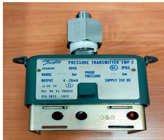
Figure 10. Example of pressure switch with ingress protection rating (IP65). Integer “6” refers to solid ingress level. (No ingress of dust; complete protection against contact dust-tight. A vacuum must be applied. Test duration of up to 8 h based on airflow.) Integer “5” refers to liquid ingress level. (Protection against water jets, water projected by a nozzle (6.3 mm (0.25 in)) against enclosure from any direction shall have no harmful effects).
