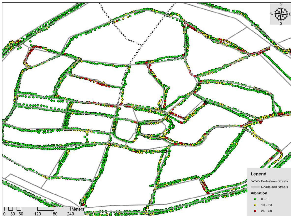
Figure 2. Vibration data from the SEE.SENSE smart bicycle lights.
