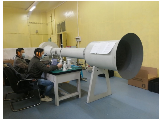
Figure 15. Wind tunnel calibration test system.
